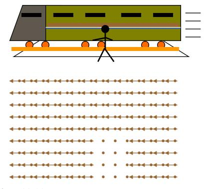
If it appears that the entire picture has shifted and that there is no distinction of subject or background, the camcorder can identify this and deduce that the cameraholder's hand has shifted. The camcorder can then compensate for the shift.
