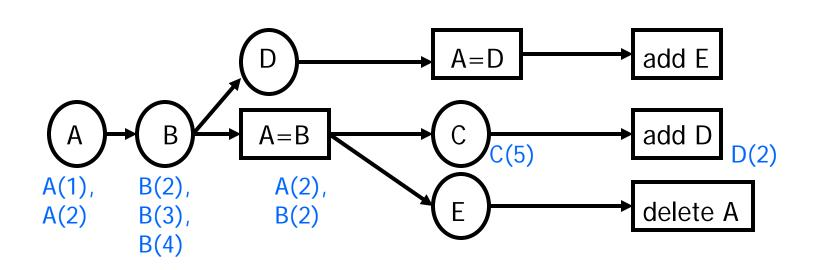
Circular nodes: fetches to WM; rectangular nodes: unifications  $A(x) \land B(x) \land C(y) \Rightarrow add D(x)$   $A(x) \land B(y) \land D(x) \Rightarrow add E(x)$  $A(x) \land B(x) \land E(x) \Rightarrow delete A(x)$
