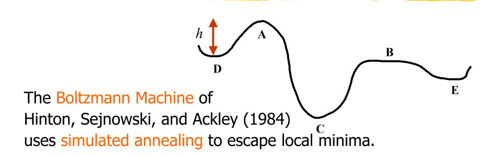
To motivate their solution, consider how one might get a ball-bearing traveling along the curve to "probably end up" in the deepest minimum. The idea is to shake the box "about h hard" — then the ball is more likely to go from D to C than from C to D. So, on average, the ball should end up in C's valley.
