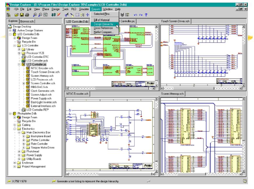
Protel's hierarchical schematic design features let you take a "bottom up" or "top down" approach, depending on your preferred methodology. Protel can automatically generate sub-sheets based on higher-level sheet symbols, or create sheet symbols based on existing sheets.
