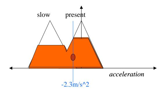
In the last step, defuzzification, we return as our acceleration Value the x coordinate of the center of mass of the merged area
