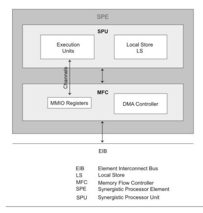
Figure 19. SPE architectural block diagram
