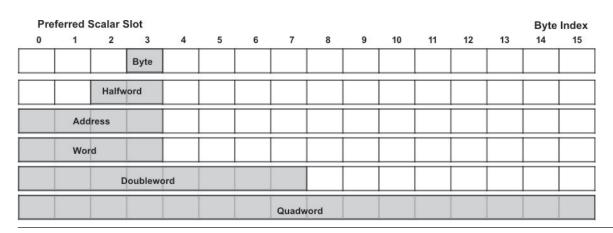
Figure 22. Register layout of data types and preferred (scalar) slot
