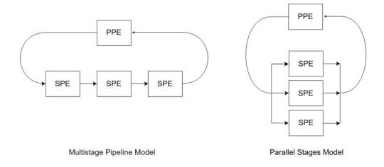
Figure 8. PPE-centric multistage pipeline model and parallel stages model
