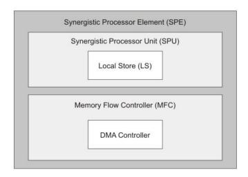
Figure 3. Synergistic Processor Element (SPE) block diagram
