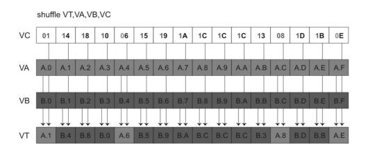
Figure 6. Byte-shuffle operation
