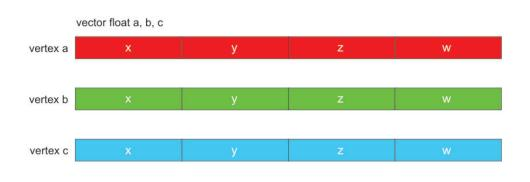
Figure 24. Array-of-structures data organization for one triangle
