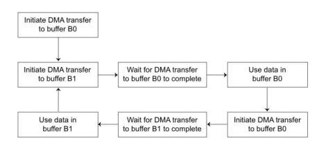
Figure 26. DMA transfers using a double-buffering method
