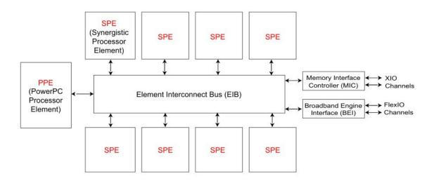
Figure 1. Overview of Cell Broadband Engine architecture
