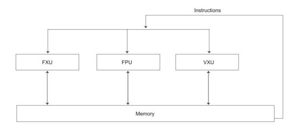
Figure 11. Concurrent execution of integer, floating-point, and vector units
