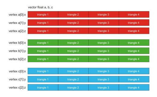
Figure 25. Structure-of-arrays data organization for four triangles
