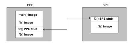
Figure 27. Example of the Function-Offload (or RPC) Model
