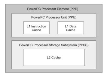
Figure 2. PowerPC Processor Element (PPE) block diagram
