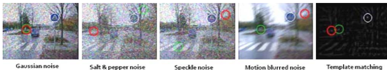
Fig. 10 Pedestrian sign detection over noisy images with biased saliency model. From left to right: Gaussian noise ( \mu = 0, \sigma = 0.5 ), salt & pepper noise ( d = 0.6 ), speckle noise with density d = 0.5 ,
