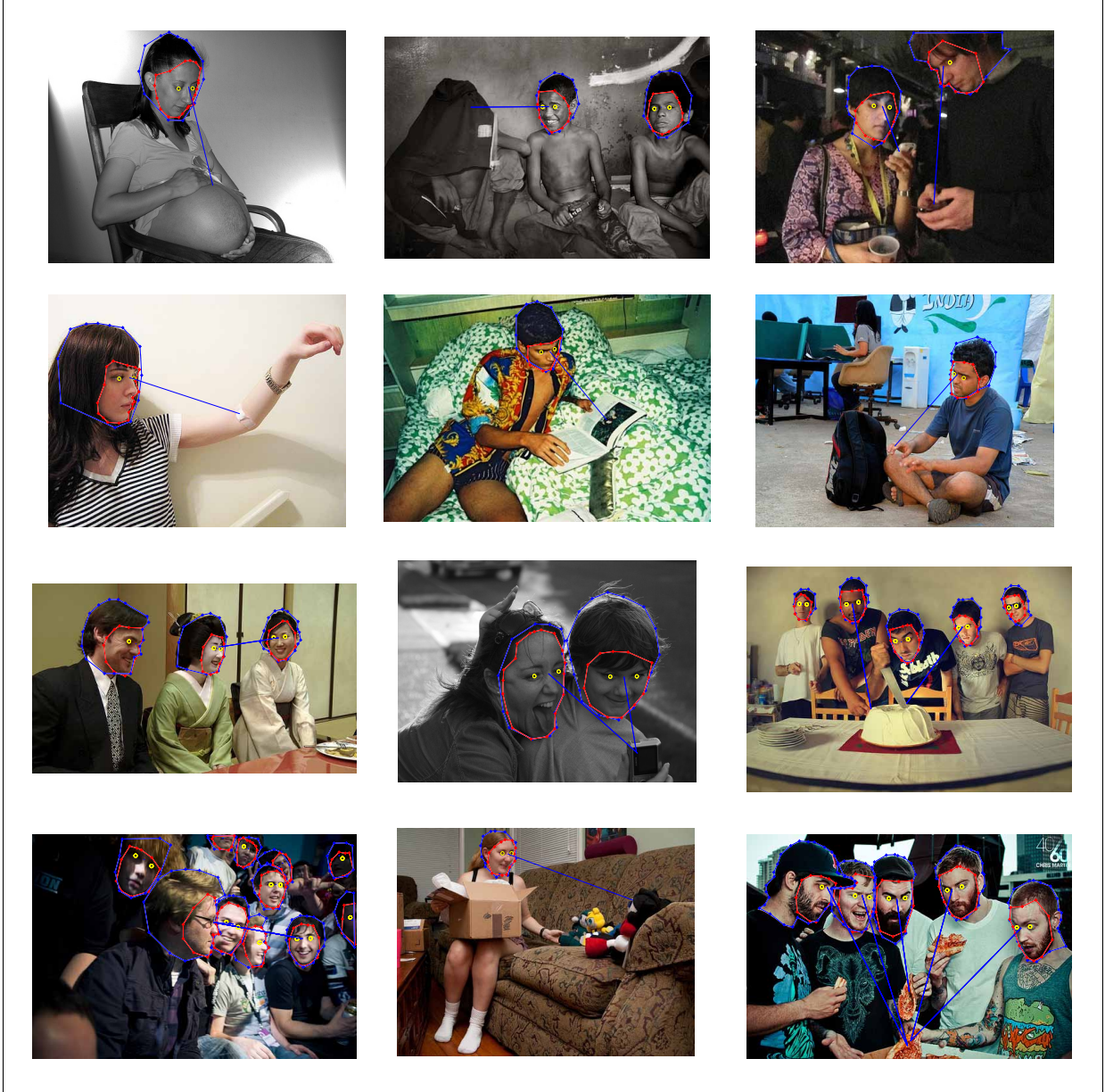
Figure 4: Sample images in the second experiment with heads, faces, eyes, and gaze directions annotated. Blue lines indicate ground truth gaze direction. We use the head region for calculating saccade pdfs. We annotated the gaze directions of the people that looked at something or a person in the scene (and not to the camera or out of the image plane). All faces were annotated.
