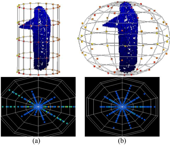
**Figure 6: 3D visual hull and the shape distribution of the surface using a cylinder (a) and a sphere (b) as reference surface.**
