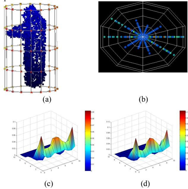
**Figure 8: Stability of the shape descriptor with regard to noisy information. (a) noisy visual hull ( $\sigma = 2$ ) and its shape descriptor (b). (c) and (d) display the polar spherical distributions for a selected radius ( $r=0.1$ ) of the noisy visual hull depicted in (a) and the original one illustrated in Figure 6.a.**
