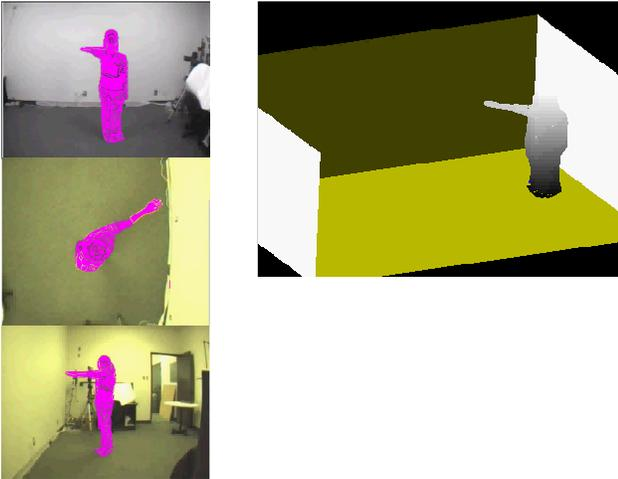
**Figure 5: 3D visual-hull reconstructed from the 3 silhouettes shown on the left**
