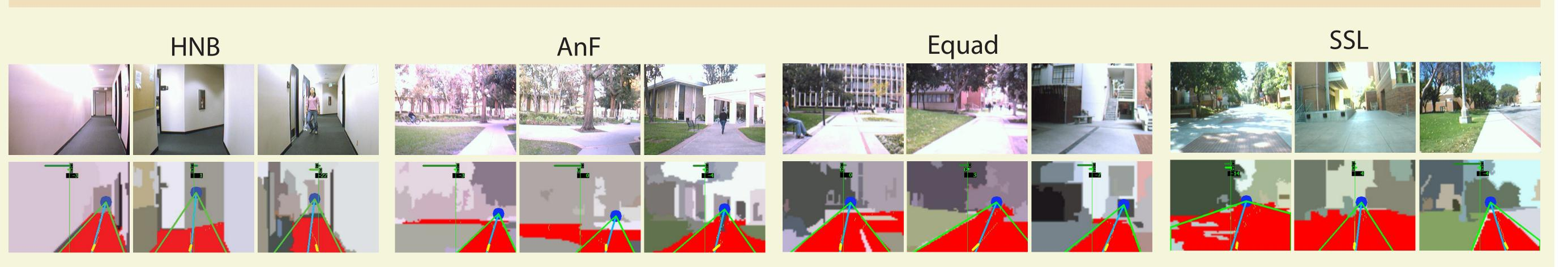
We selected various indoor and outdoor to test the system's robustness against lighting, road appearance and size, as well as obstacles in a form of walking pedestrians.
