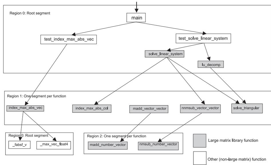
Figure 16. Large matrix overlay program call graph
