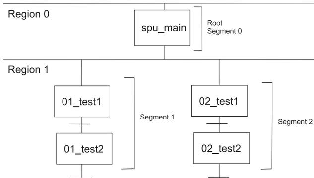
Figure 12. Simple overlay program regions, segments and sections
