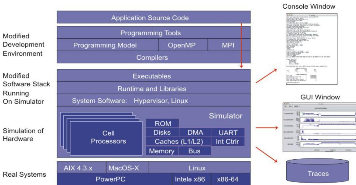
Figure 28. Simulation stack
