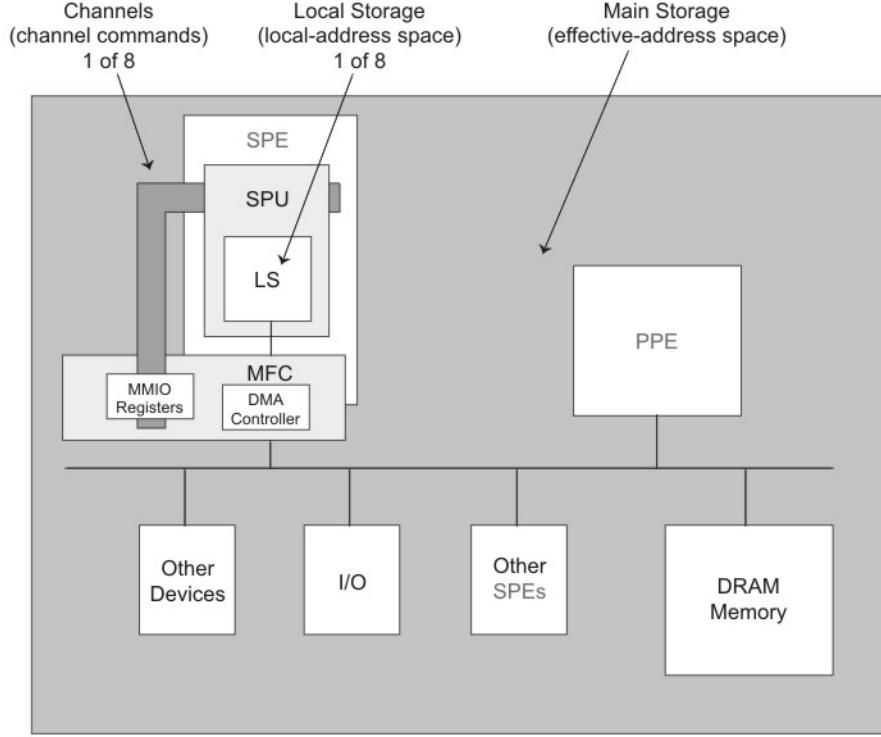
*Figure 13. Storage domains defined in the Cell Broadband Engine*
