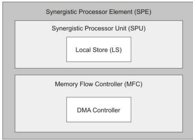
*Figure 3. Synergistic Processor Element (SPE) block diagram*
