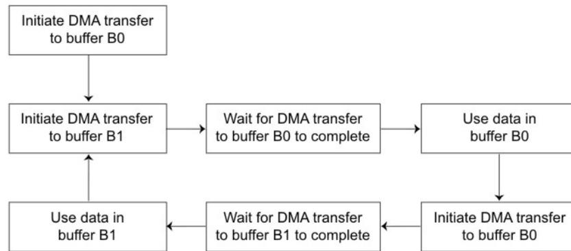
Figure 26. DMA transfers using a double-buffering method
