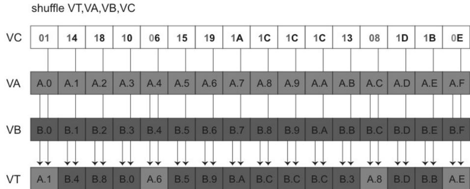
Figure 6. Byte-shuffle operation
