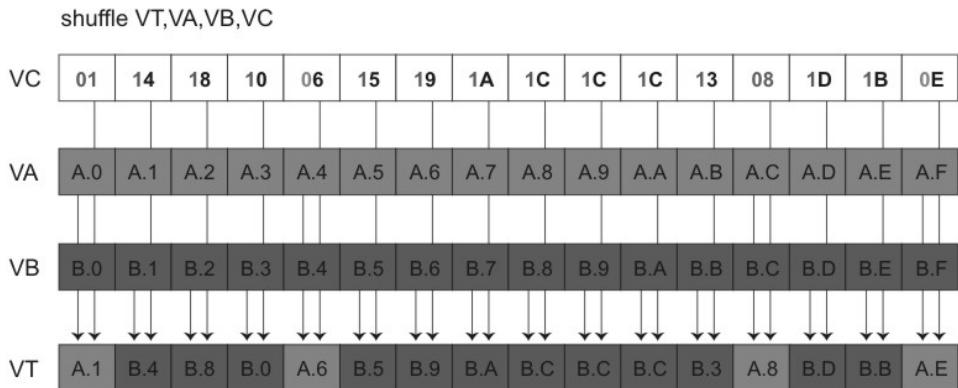
*Figure 6. Byte-shuffle operation*
