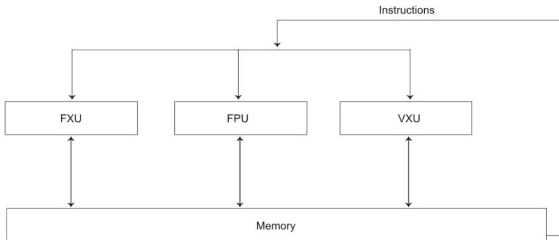
Figure 11. Concurrent execution of integer, floating-point, and vector units
