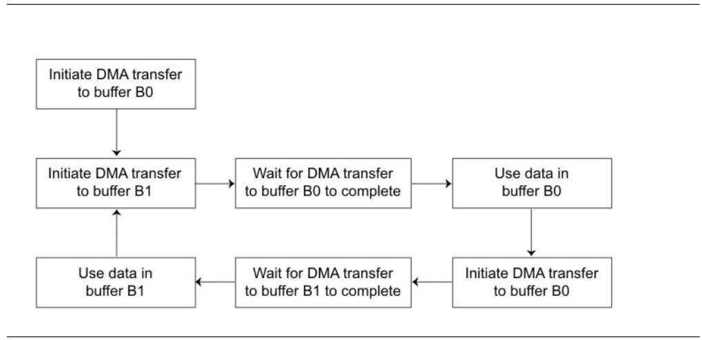
Figure 26. DMA transfers using a double-buffering method
