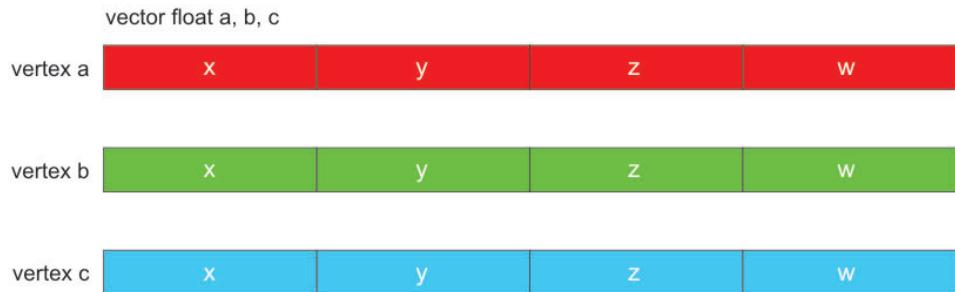
Figure 24. Array-of-structures data organization for one triangle
