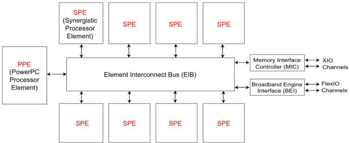
Figure 1. Overview of Cell Broadband Engine architecture
