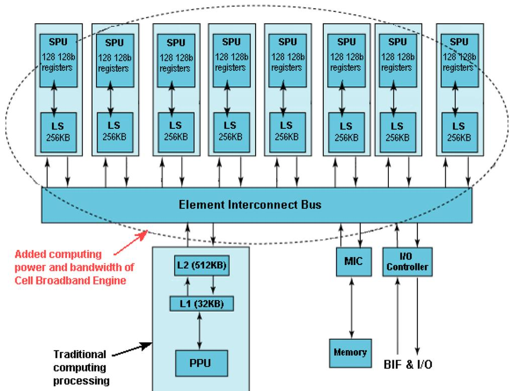
At the heart of the new multiprocessor is the PowerPC® Processor Unit (PPU). The PPU is a 64-bit processor fully compliant with the Power Architecture™ standard, and capable of running both operating systems and applications. The multiprocessor also incorporates a set of eight Synergistic Processor Units (SPUs) into its design. The SPUs are optimized for running computationally intensive applications, operate independently of each other, and can access memory shared between all SPUs and the PPU.
