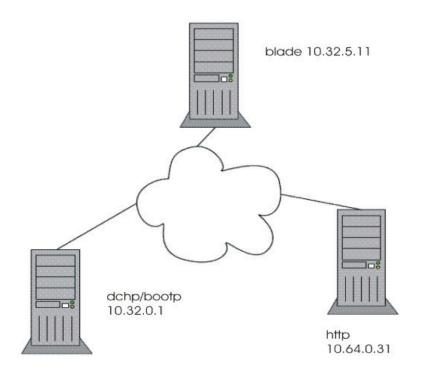
Figure 1. The network installation environment
