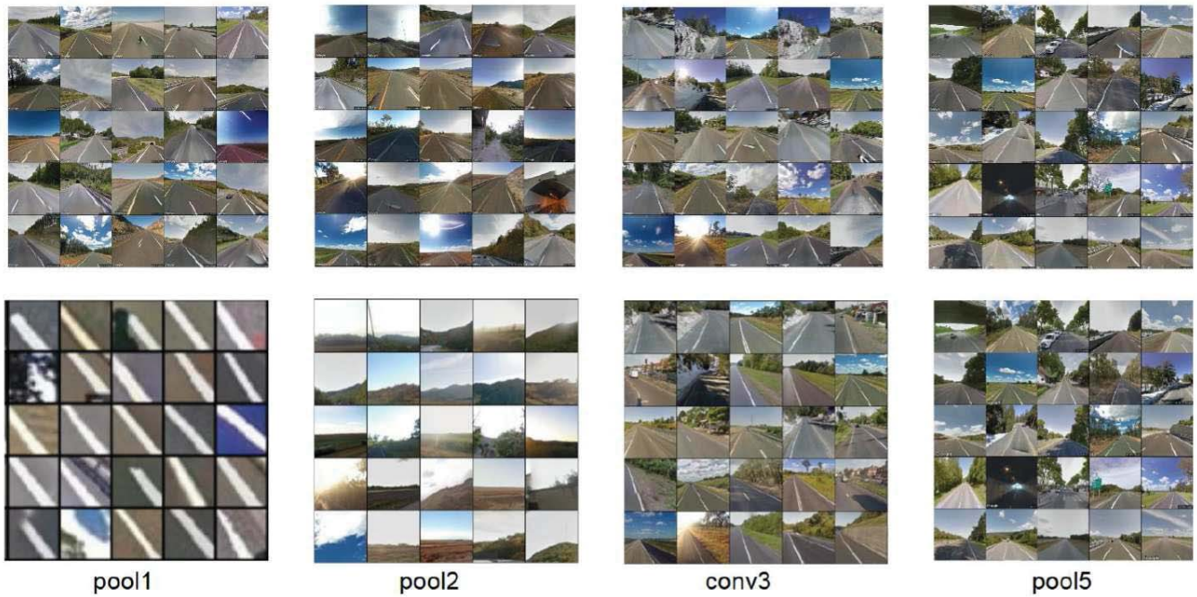
Fig. 9. Visualization of receptive fields of filters at different layers. Top : top 25 images with the strongest activations for filters at a few layer (pool1, pool2, conv3, and pool5); Bottom : 25 image patches from the corresponding images on the 1st row, that excite the filter the most.
