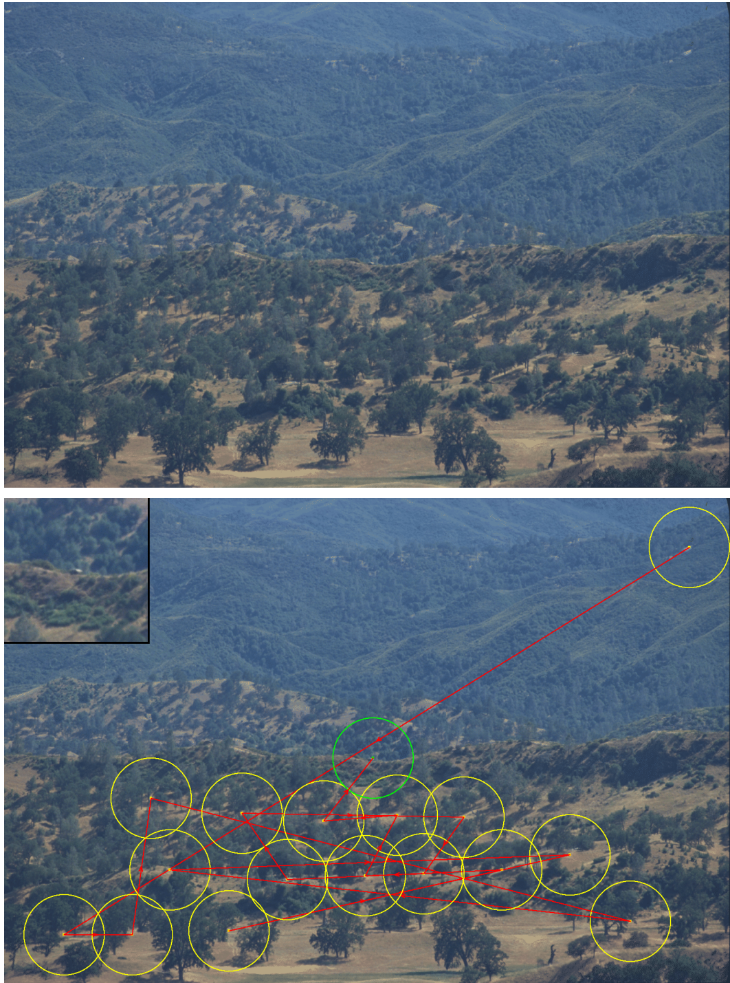
Figure 3.13: A more difficult example from the image database of military vehicles. (Top) The input color image. Humans found the location of the vehicle in 7.5 sec. on average. (Bottom) The target is not the most salient object, and the model searches the scene in order of decreasing saliency. The algorithm came to rest on the location of the target on the 17 th shift, after 6.1 sec (using same time scaling as in the previous figure).
