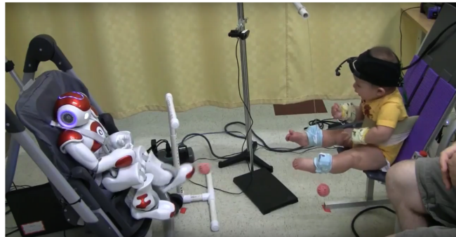
Fig. 1. Experiment setup of the SAR leg movement study; the infant is seated across from the Nao robot and is wearing leg and arm motion trackers and an eye tracker. This work uses data from the study to explore Bayesian surprise as a potential predictor of infant visual attention.
