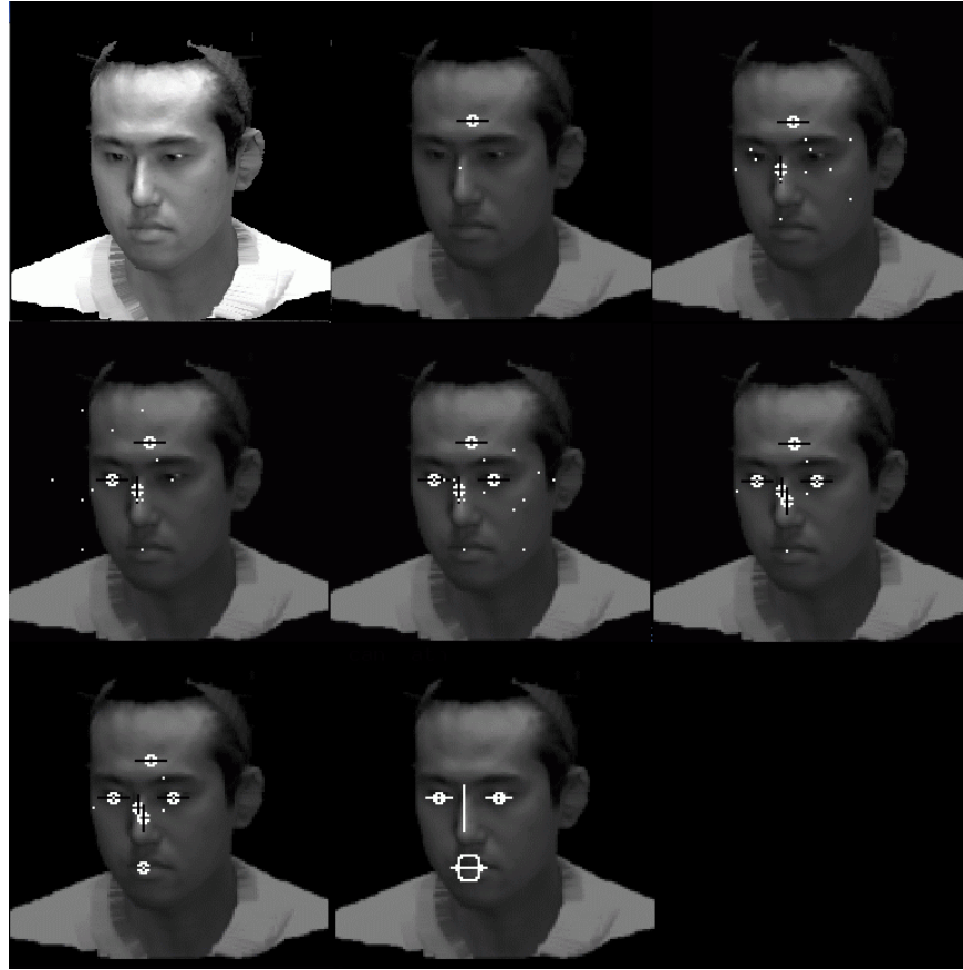
Figure 6: Step by step detection of a face.
