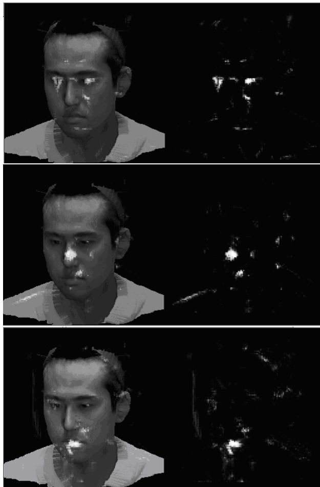
Figure 5: The resulting neural network based eye, nose and mouth detector
