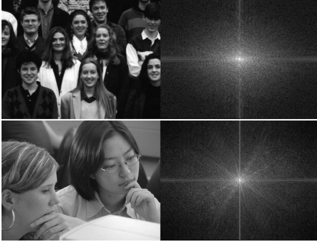
Figure 2: images with their corresponding Fourier Transform
