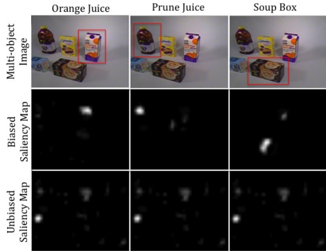
Fig. 2. Example of top-down attention biasing. Red boxes surround desired objects, to which attention has been focused in the biased saliency map, as compared to the unbiased saliency map, which highlights all salient objects equally.
