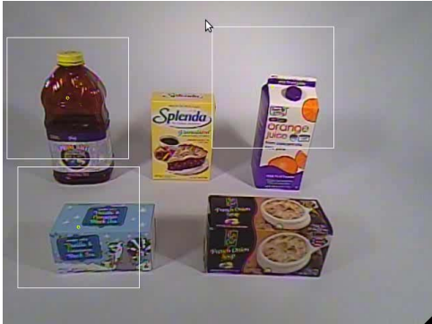
Fig. 7. Example 5-object image with the 3 most salient attention-biased regions (biased based on the user's query of orange juice) shown in white rectangles.
