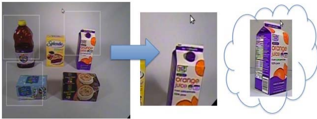
Fig. 8. SURF object recognition applied to 3 rectangles chosen by attention biasing; the best rectangle (right of blue arrow) was chosen based on the closest match to the database instance (depicted in the cloud) of the user query for orange juice.
