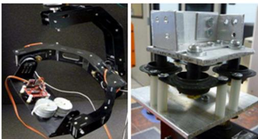
Fig. 8: PS1-3X Camera Gimbal with IMU (left), cluster of 4 vibration isolators to damp vibrations (right).
