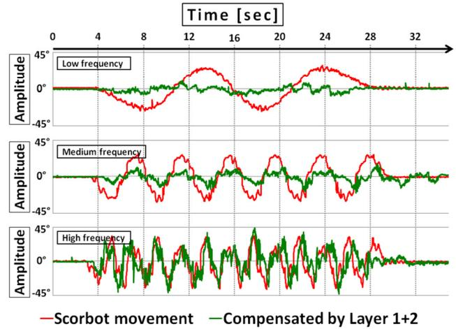
Fig. 11: Layer 1+2 achieve good results for low/medium frequency vibrations. No improvement for high frequency vibrations.
