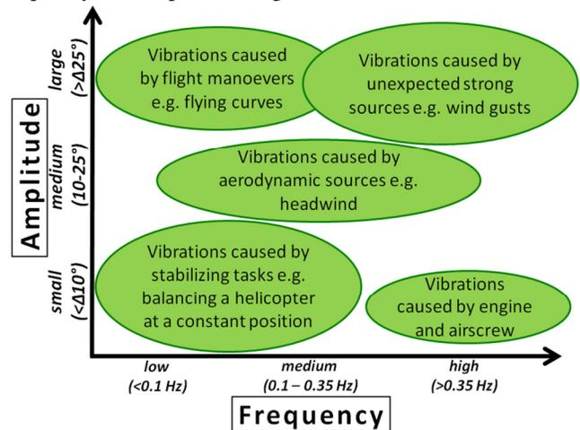
Fig. 2: Sources of vibrations in aerial robotics [7].
