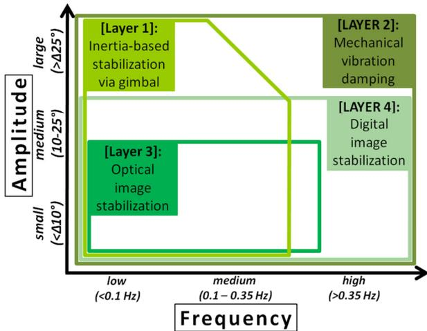
Fig. 3: The combination of four stabilization techniques in the VISS architecture covers the entire frequency-amplitude spectrum of vibrations.
