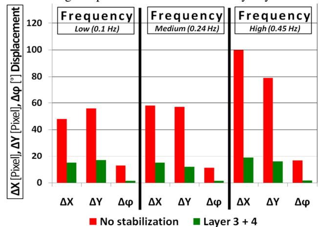
Fig. 12: Results of basic functionality test: Performance of Layer 3+4 was determined based on horizontal, vertical, and angular displacement.
