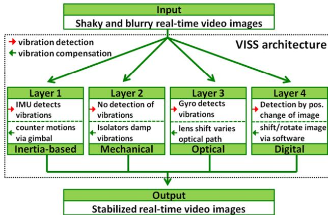
Fig. 4: The VISS architecture combines four layers. Each layer represents a self-contained stabilization technique which covers vibrations of Fig. 2.
