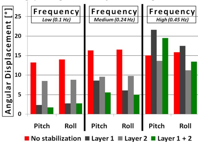
Fig. 10: Results of basic functionality test: Performance of Layer 1 and 2 along pitch and roll axis was tested separately and in combination.
