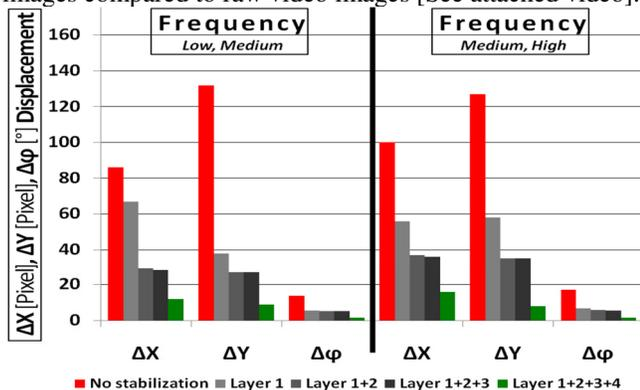
Fig. 13: Two UAV-flights with displacements measured layer by layer: Left: (low/medium freq.) Final error: 12 pixel (X), 9 pixel (Y), 1.5° (φ). Right: (medium/high freq.) Final error: 16 pixel (X), 8 pixel (Y), 1.6° (φ).
